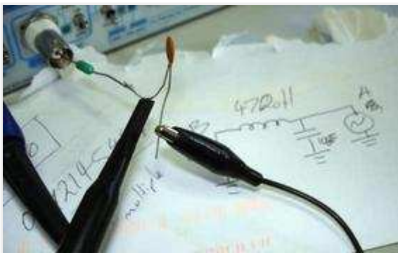
Fig [9] - "Back of an Envelope" Tank Circuit
