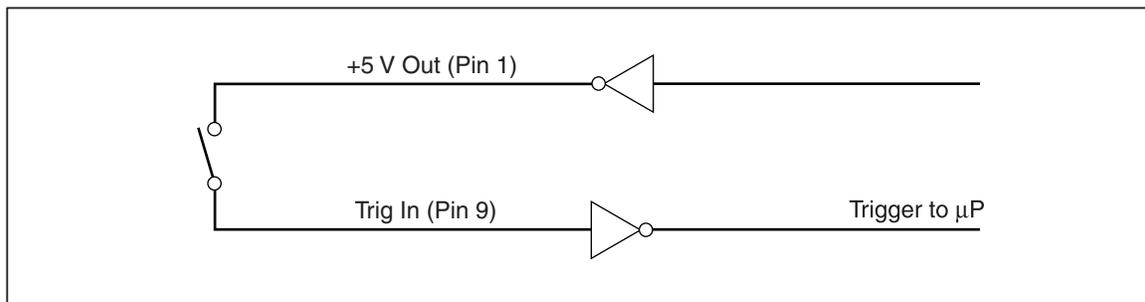
**Figure 4-1. External Trigger Using Pin 9 of RS-232 Interface**
