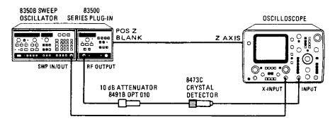
Connect the equipment listed above as shown in the above diagram. Select External Sweep on oscilloscope.
