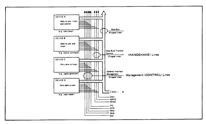
Figure 3-5. Interface Connections and Bus Structure
