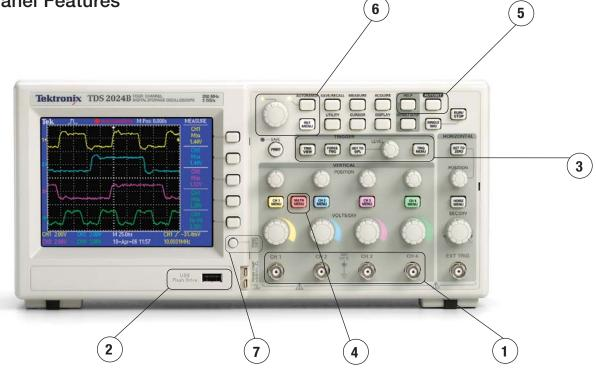
1 Digital Real-Time Technology – Quickly debug and characterize a wide range of signal types on four channels simultaneously with Tektronix' unique digital real-time (DRT) sampling technology. This acquisition technology allows you to capture high-frequency, non-repetitive information, such as glitches and edge anomalies, that eludes other oscilloscopes in its class.
